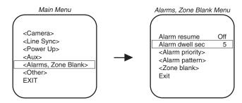
This is the minimum time the Spectra II will stay at an alarm even if the alarm is present for less than this amount of time.
